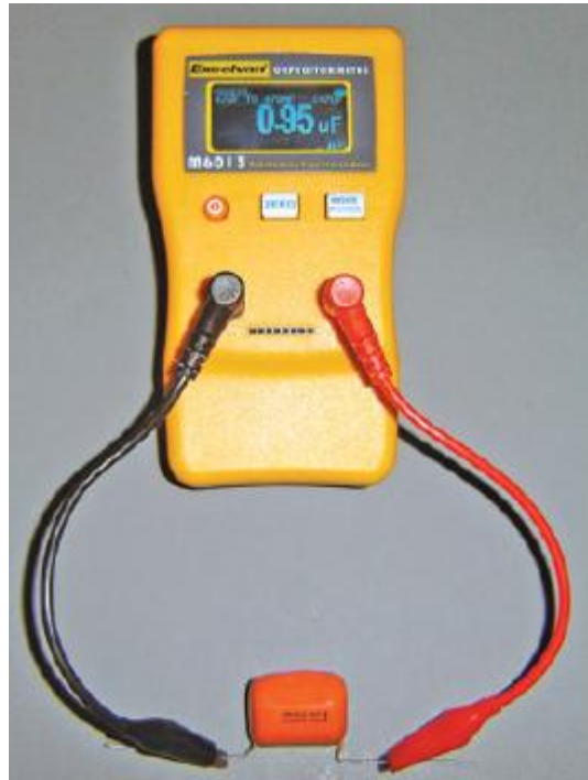
Figure 14 M6013 Capacitor Meter
